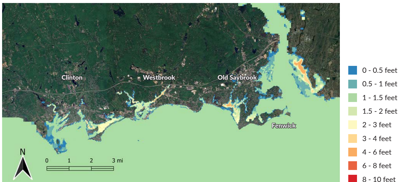
Figure 3-17: Tidal Simulation Water Depth Difference Between 2070 Sea Level Rise and Existing Conditions
