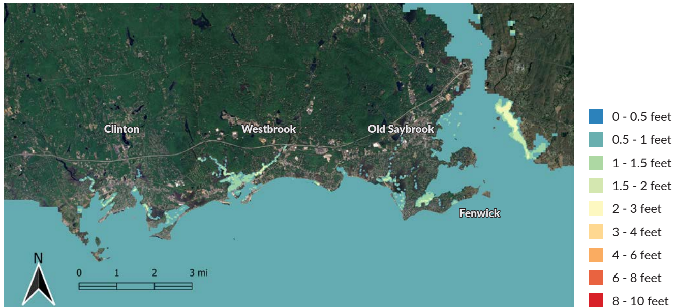
Figure 3-16: Tidal Simulation Water Depth Difference Between 2050 Sea Level Rise and Existing Conditions
